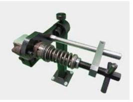
Clamp installation pump section DAF Bosch 0414755005
