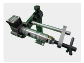
Clamp installation pump section MV ATEGO
