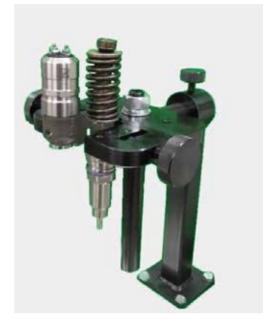
Clamp installation injector pump SCANIA
