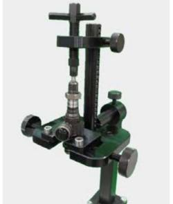
Clamp installation injector pump SCANIA H-shaped
