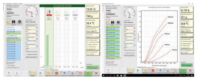
The software has a user-friendly interface. The program contains built-in test plans for testing and coding Bosch, Delphi, Denso, Siemens (VDO) injectors. Functions for creating new test plans, editing built-in ones, as well as creating targets for Delphi C2i, C3i, C4i injectors are available. The results and progress of testing are displayed in graphical form and saved to a file and sent to print.
