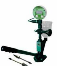
DL-RP410(without pressure sensor)DL-RP415(with pressure sensor. 1500 bar)
