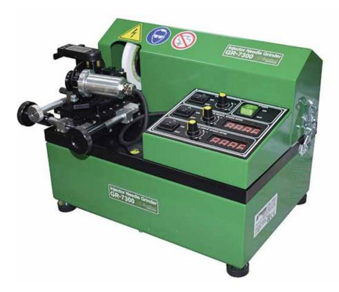
The **DL-GR7300** machine is used for sharpening needles of atomizers and other bodies of rotation. The machine is controlled by PWM controllers.
