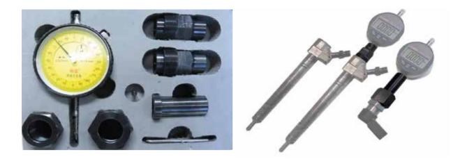
Adapter set with indicator head for measuring valve travel CR VDO Siemens injectors of all types.
