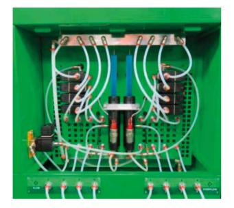
Liquid flow meter for simultaneous checking from 1 to 4 nozzles. Installed on a stand.
