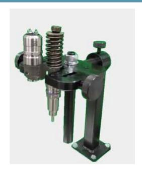
Clamp installation injector pump SCANIA
