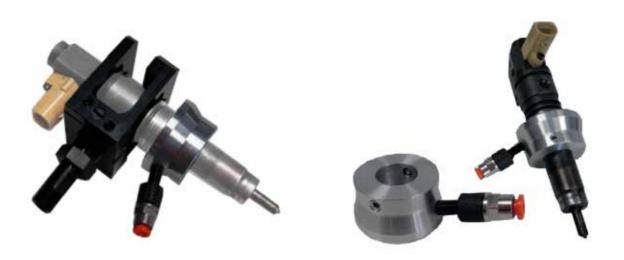
Installation in nozzle adapter Delphi Smart with direct "0°" approach.
