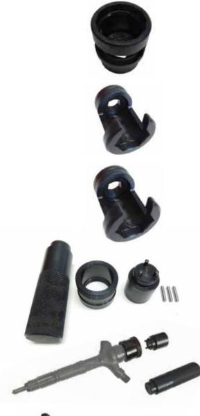
Wrench for dismantling the injector solenoid DENSO, CAT, PERKINS Key Features:
