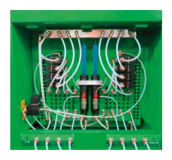
Liquid flow meter for simultaneous checking from 1 to 4 nozzles. Installed on a stand.
