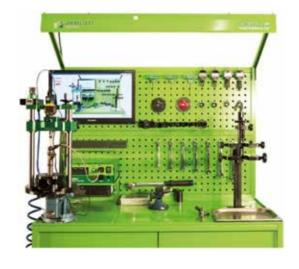
Clamp for disassembly-assembly of injectors.
