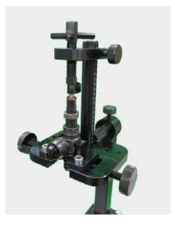
Clamp installation unit injector AUDI / VW 1.9
