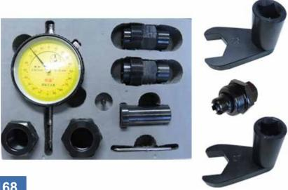
Set of adapters and wrenches for repairing CR VDO Siemens injectors
