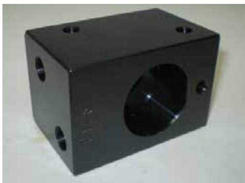
Clamp for Volvo FH12 and some Iveco injectors from Bosch CB0124-01
